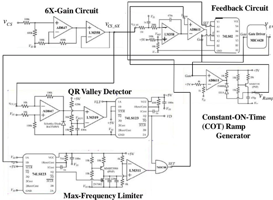
**Figure-18: Control circuit for QR valley switching**
