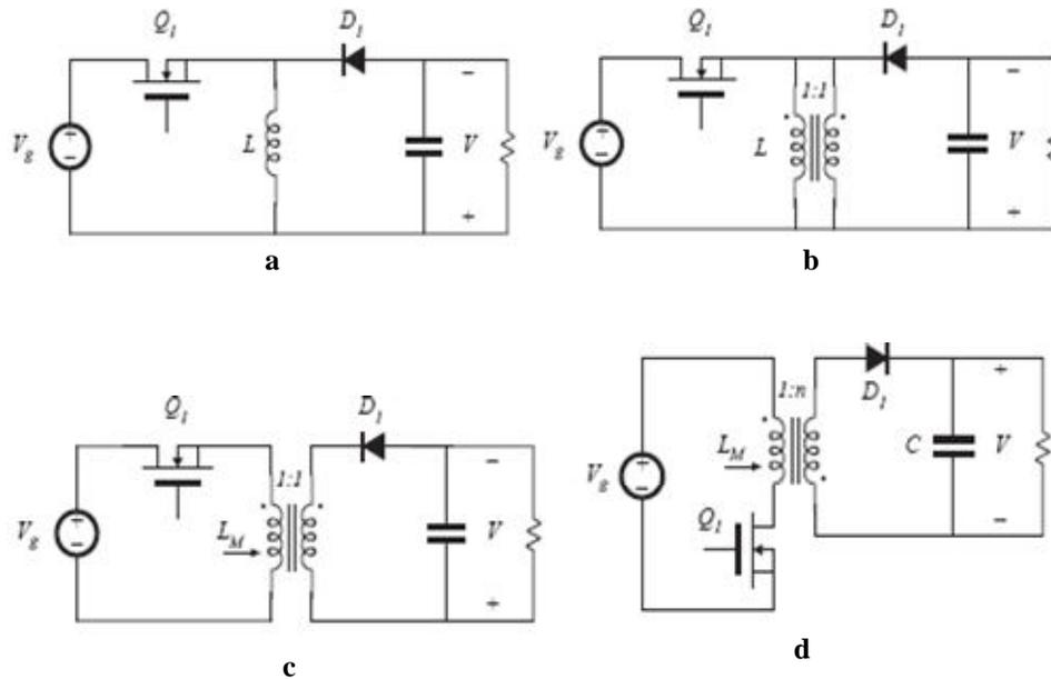
**Figure-4: Fly-Back Converter derivation**
