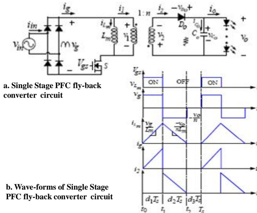
**Figure-9: Single-stage Transformer Isolated fly-back converter and its wave-forms**
