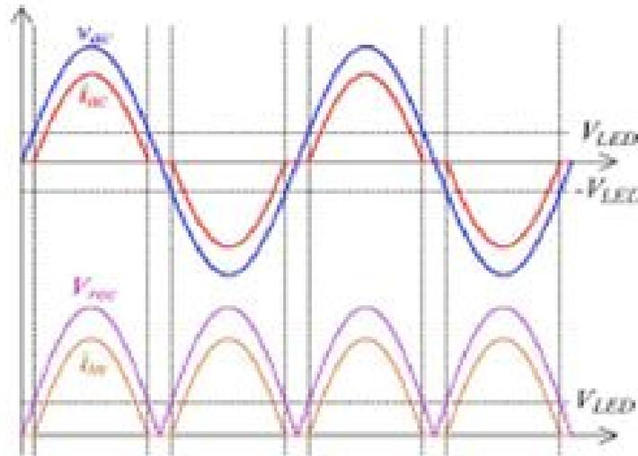
**Figure-16: Theoretical input waveforms of voltage and current**
