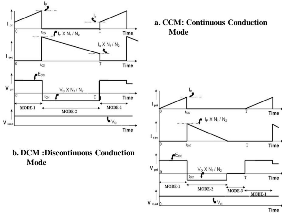
**Figure-3: Continuous & Discontinuous Modes of Operation of Fly-Back Converter**
