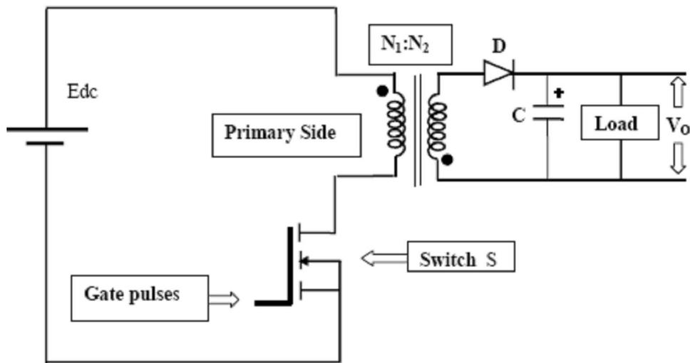
**Figure-1: Fly-Back Converter Circuit**
