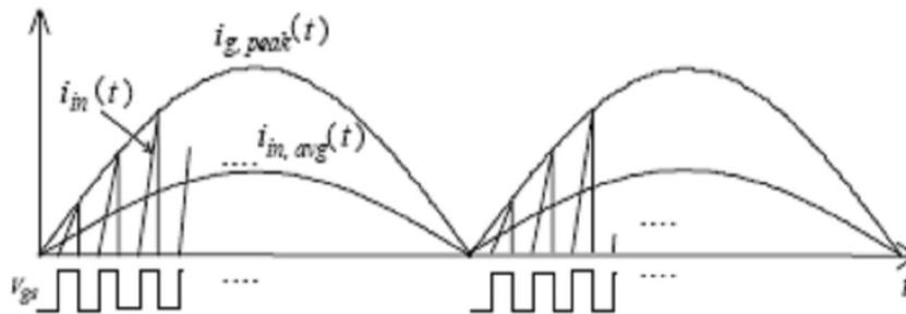
**Figure-11: Rectified Input Current Wave-form of the Fly-Back Converter**
