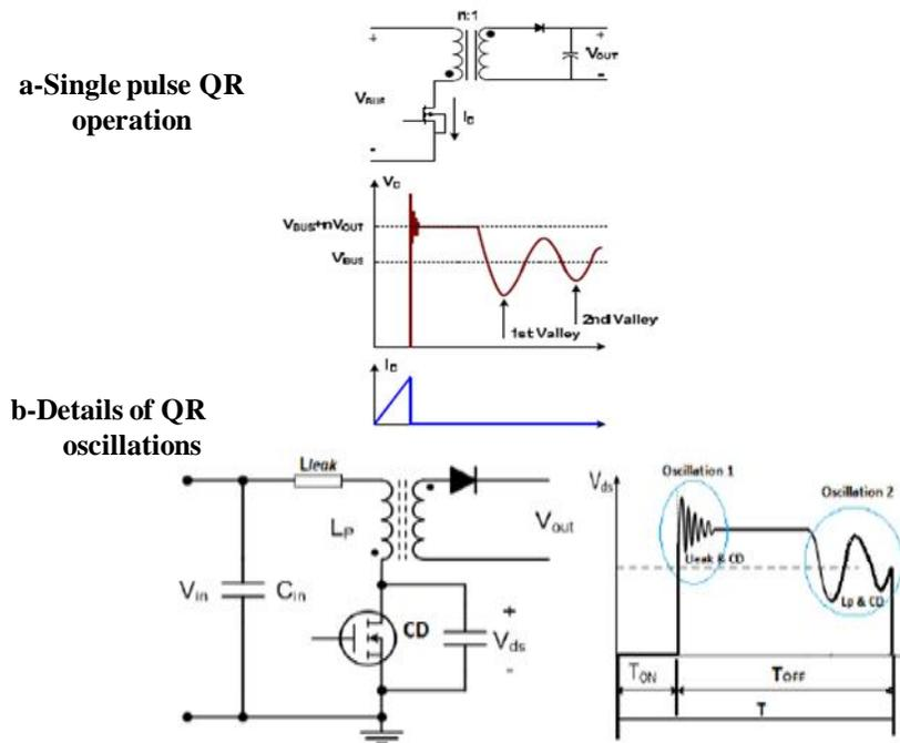
**Figure-19: Single pulse of Fly-Back Converter showing Quasi Resonance Oscillations**
