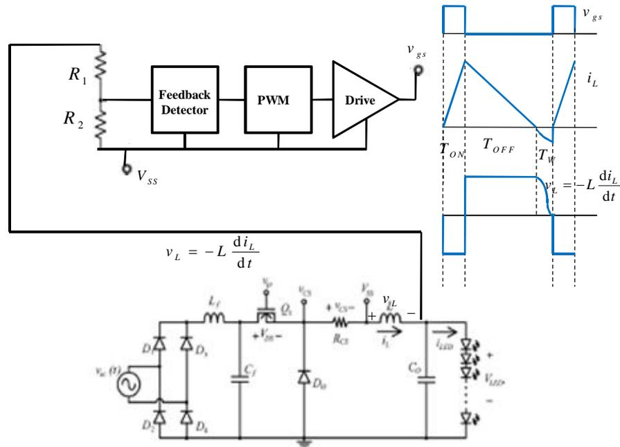
**Figure-21: QR Valley switching from inductor voltage sensing**
