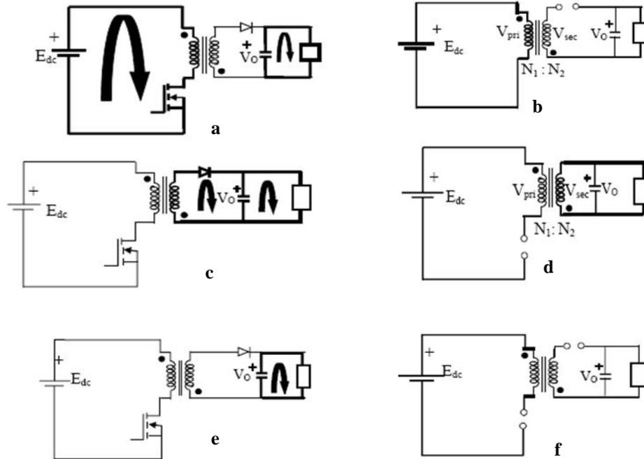
**Figure-2: Modes I, II and III operations of Fly-Back Converter**
