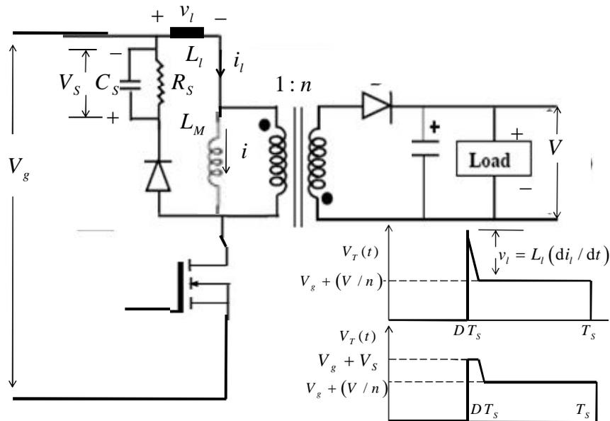
**Figure-8: Use of SNUBBER Circuit**
