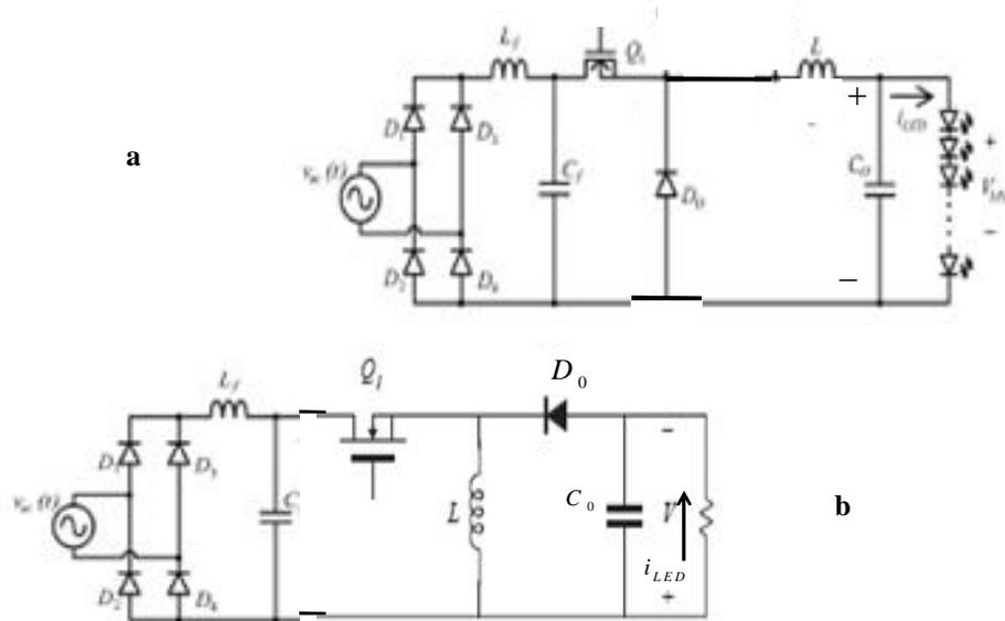
**Figure-12: Configuration of buck-converter with one-inductor**
