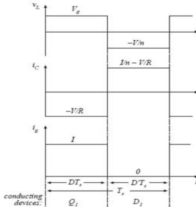
**Figure-6: Fly-Back Converter Average or DC Wave-Forms Continuous Conduction Mode**
