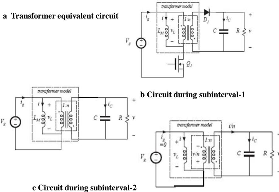
**Figure-5: Fly-back converter circuit during operation at different subintervals**
