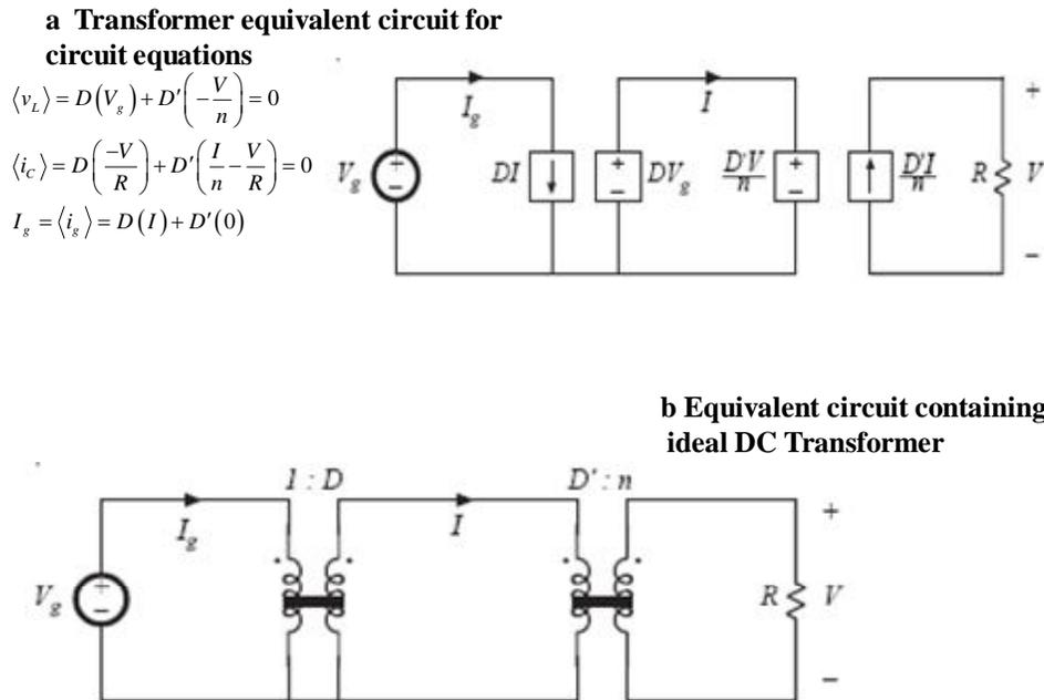
**Figure-7: Fly-Back Converter Equivalent Circuit Model Buck-Boost System**
